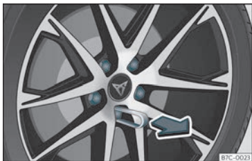
Fig. 35 Wheel: wheel nuts with caps.
