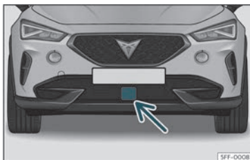
Fig. 140 On the front bumper: radar sensors.
