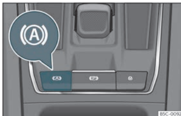
Fig. 168 In the lower part of the centre console: Auto Hold function button.
