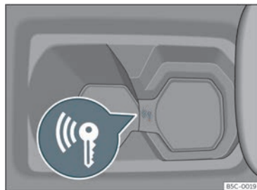
Fig. 135 In the centre console: emergency start. »
