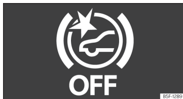
Fig. 150 On the instrument panel display: Front Assist deactivated indication.
