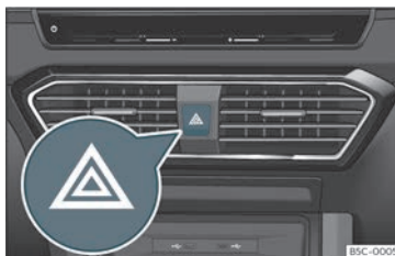
Fig. 87 Dash panel: hazard warning lights switch
