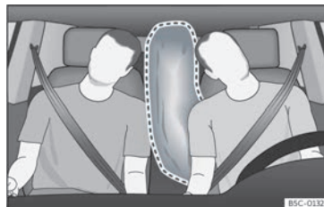
Fig. 20 Fully inflated central airbag (deployment zone).
