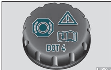
Fig. 190 Engine compartment: brake fluid reservoir cap.
