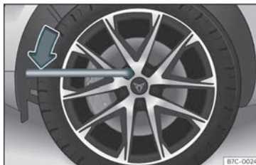
Fig. 37 Wheel change: loosen the wheel nuts.
