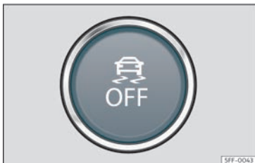
Fig. 169 In the lower part of the centre console: button to switch the ESC off/on
