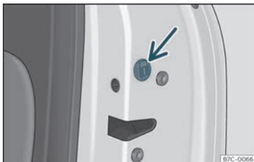
Fig. 75 Locking the door manually.
