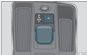
Fig. 137 In the centre console: selector lever.
