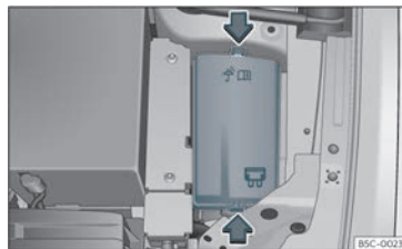
Fig. 48 In the engine compartment: fuse box cover.
