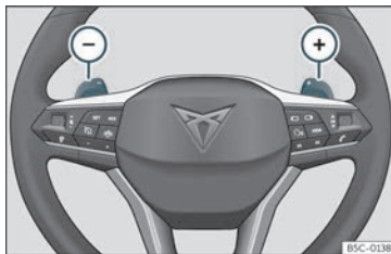
Fig. 138 Steering wheel: automatic transmission levers
