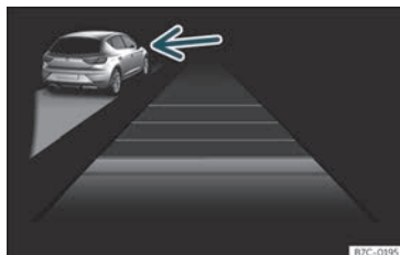
Fig. 153 On the instrument panel display: ACC active, vehicle detected in an outer lane.
