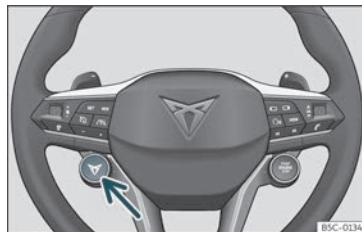
Fig. 139 Multifunction steering wheel*: button to change the driving profile.
