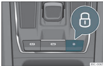
Fig. 71 In the centre console: central locking switch
